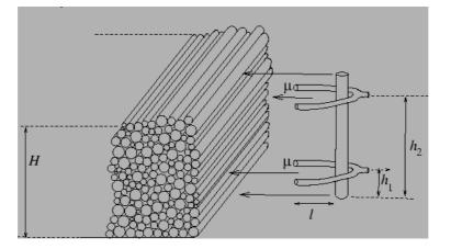
Another strong bough is put through the branching vertically (see Fig.) and fixed temporarily; then the two branches of the Y are loaded in several layers with further logs. The vertical bough passes through two Ys, which, due to weight and friction, get stuck in the stack.
