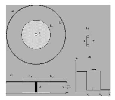
For the radii drawn in the figure  $r \ll R_1 \ll R_2$  holds. Poorly conducting material is used for the ring between  $R_1$  and  $R_2$ , while the middle ring  $(R_1)$  and the thin rim surrounding  $R_2$  conduct excellently. (The latter one is used for the inflow of the current.)
